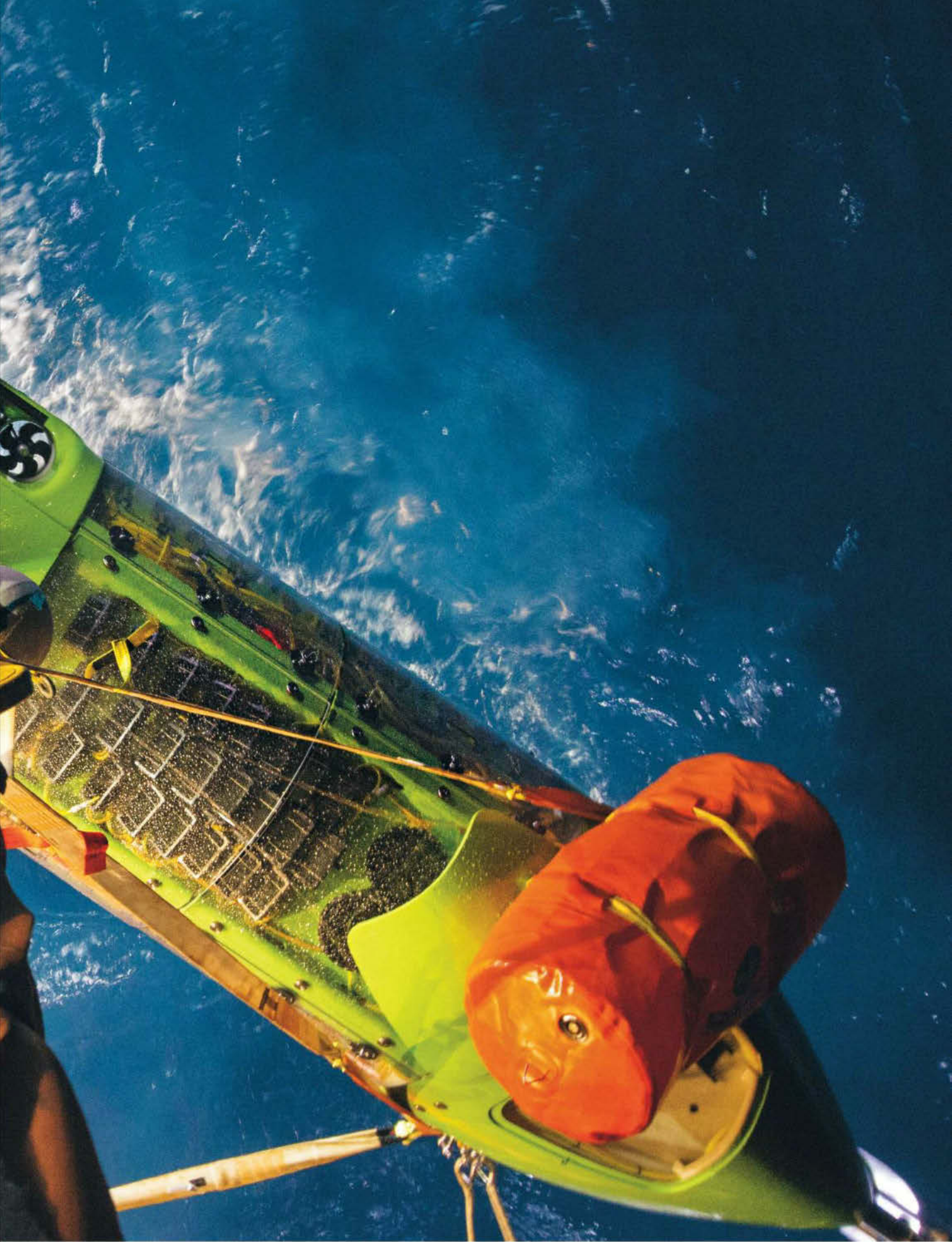
DEEPSEA CHALLENGER is lifted on deck by a shipborne crane after a test dive to 26,972 feet. The orange bag adds buoyancy for the ascent; the gray ones shift the sub to a horizontal position for recovery.
